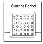
for the first period will be shown in the flashing Current Period column of the LED display. The speed settings for the next three periods will be shown in the three columns to the right.
